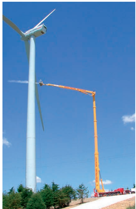
Fig. 4. S 112 HLA has the working outreach of 33 meters.
