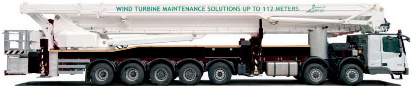
Fig. 1. The first S 112 HLA is mounted onto a Mercedes Benz 76.60 all-wheel drive chassis with 5 steered axles.
