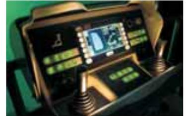
Standard even for the smallest types: operating console with high-definition TFT colour screen
